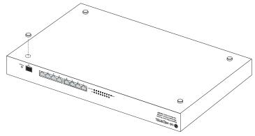
Figure 3-4 Attaching the Adhesive Feet
